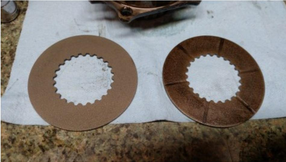
Stack it all up in same order you took it out with your new friction plates and bolt cover on with new bolts. Place Assembly in with the carriers and bolt carriers back on. Put your output shafts back in. Seal up the rear cover with RTV and bolt back on.
