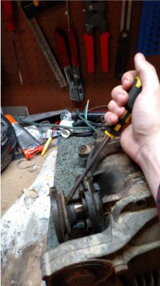
Next remove the carriers by removing the six 13mm bolts on each side.
