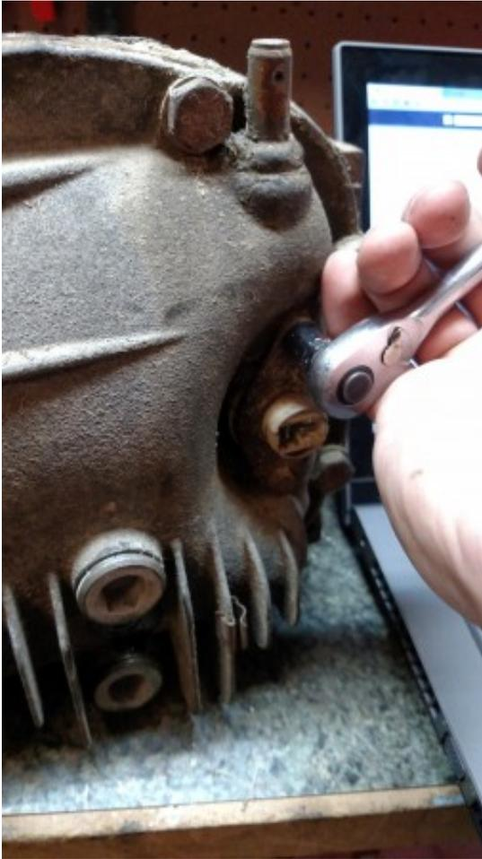
Drain the gear oil 2 17mm oil drain plug Allen key style(smelly) and remove diff cover
