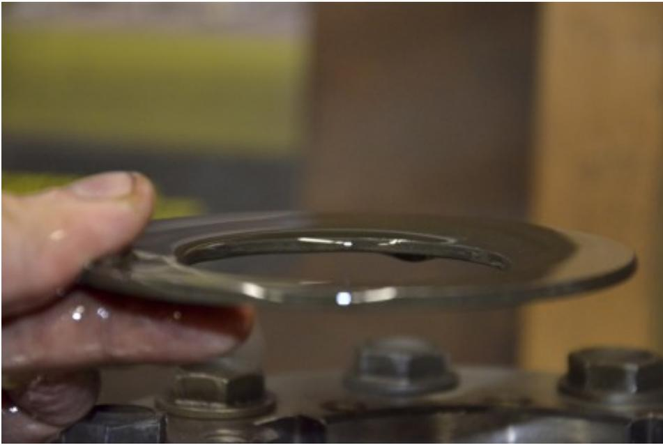
Here is the first dog ear. For me I will be reversing the way this is facing so I marked this side to face down. New dog ears go in however you want. Just under this is the first friction plate.
