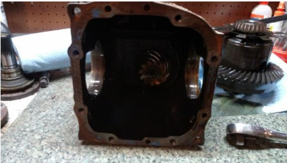
The assembly itself. Starting from the top you have the carrier bearing. Can be replaced but requires pullers and presses. I opted to skip that. the big throwing star thing is the
